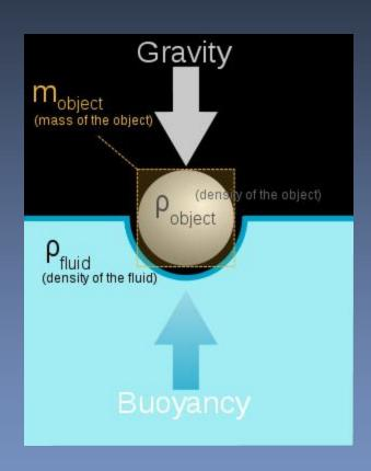
Any floating object displaces its own weight of fluid.
