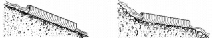
Poor design profile (vertical alignment)
